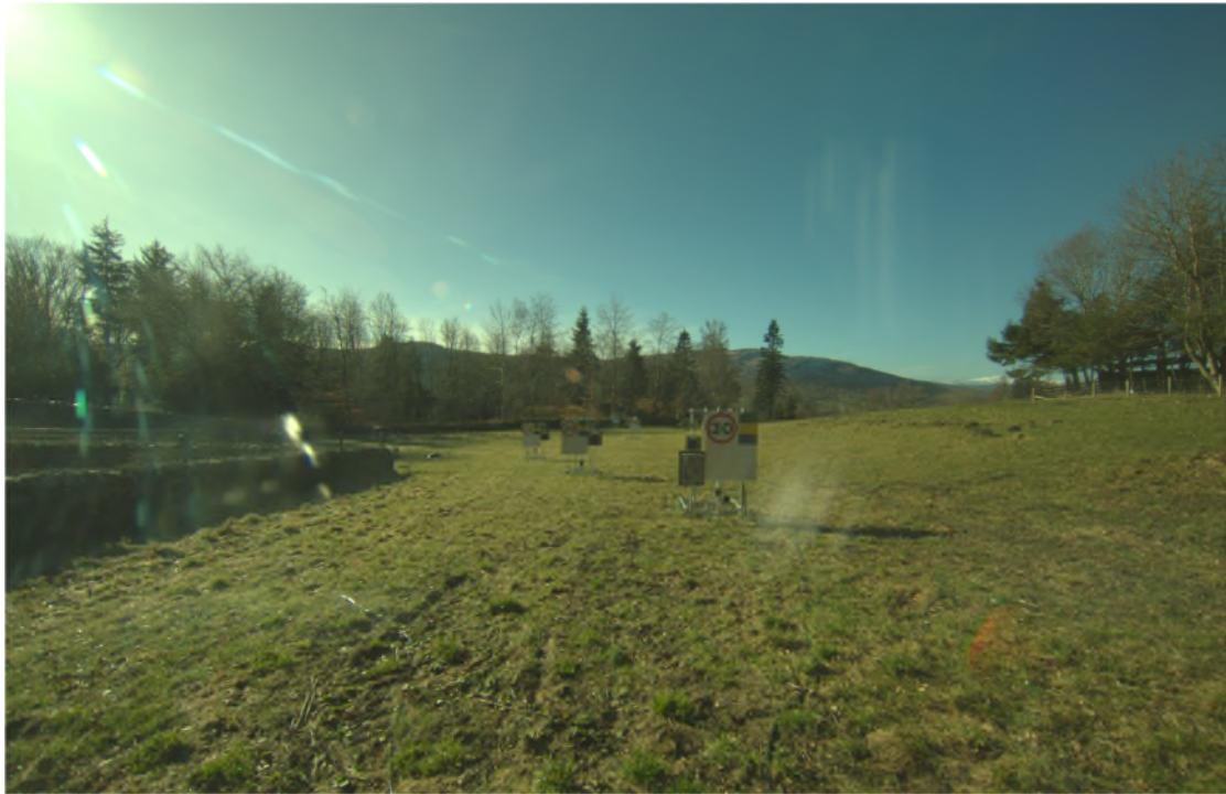
Figure 12: The sun is causing lens flare (1 March, 11:45).
