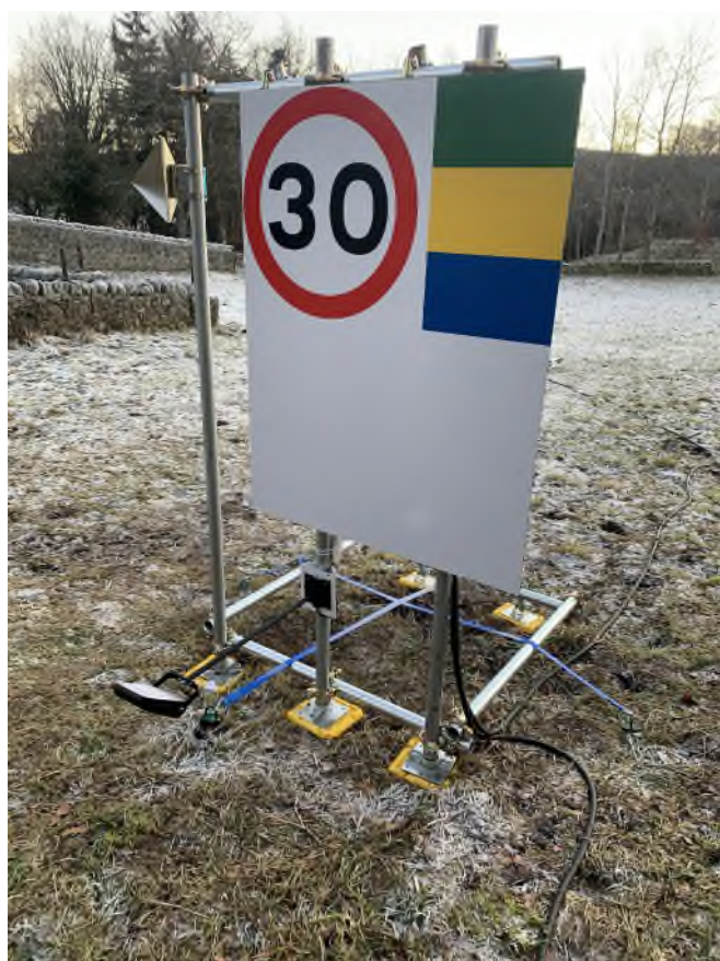
Figure 4: Custom designed sensor target.
