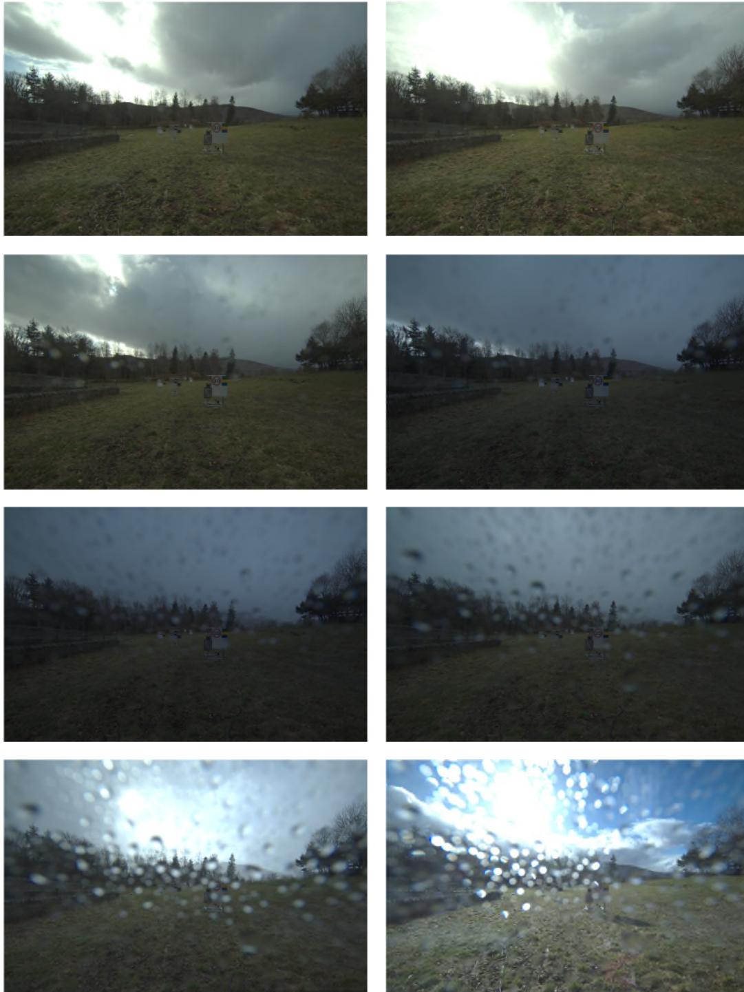
Figure 16: Light rain causing droplets on the sensor enclosure (29 Feb, 13:20-13:55).
