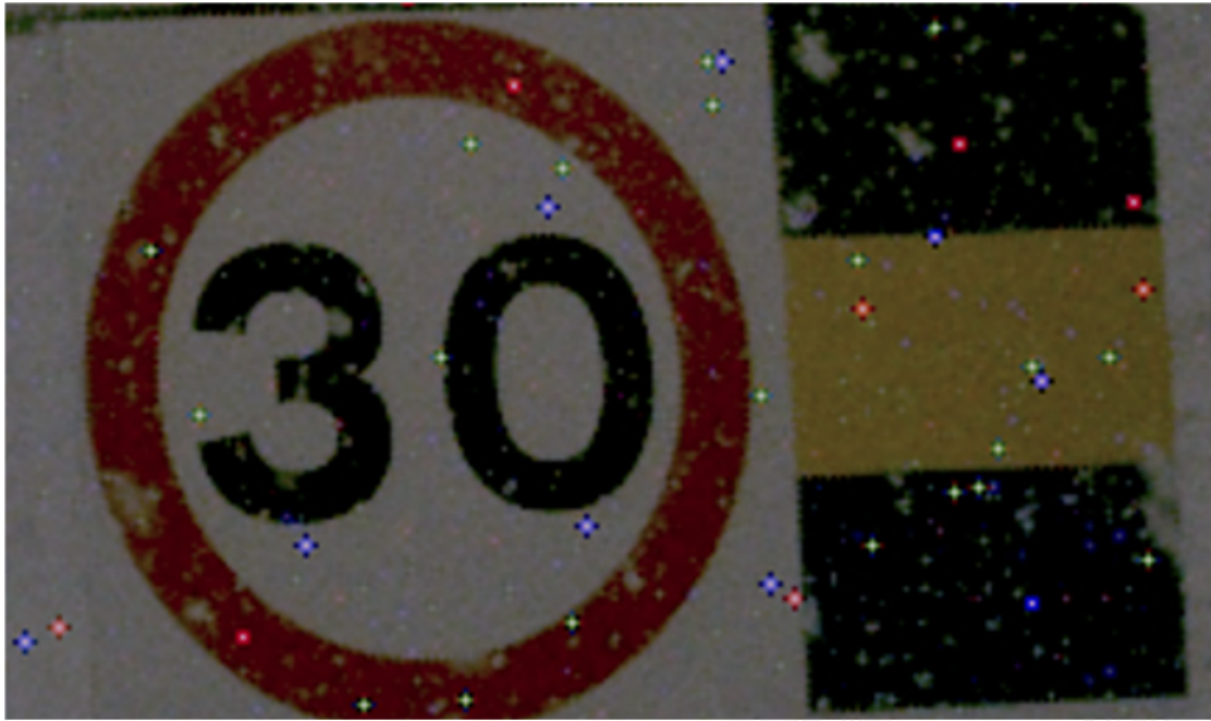
Figure 27: Moderate to Heavy Snow with visible snowflakes in front of the target (zoomed in).
