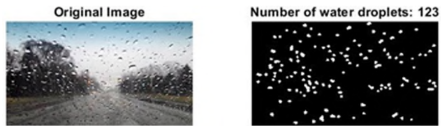
Figure 15: Canny Edge Detection with Morphological Operations.
