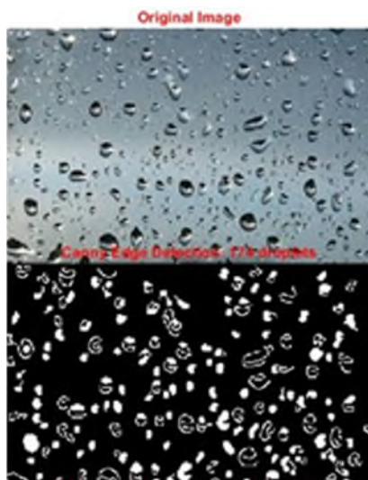
Figure 12: Canny Edge Detection simpler example.
