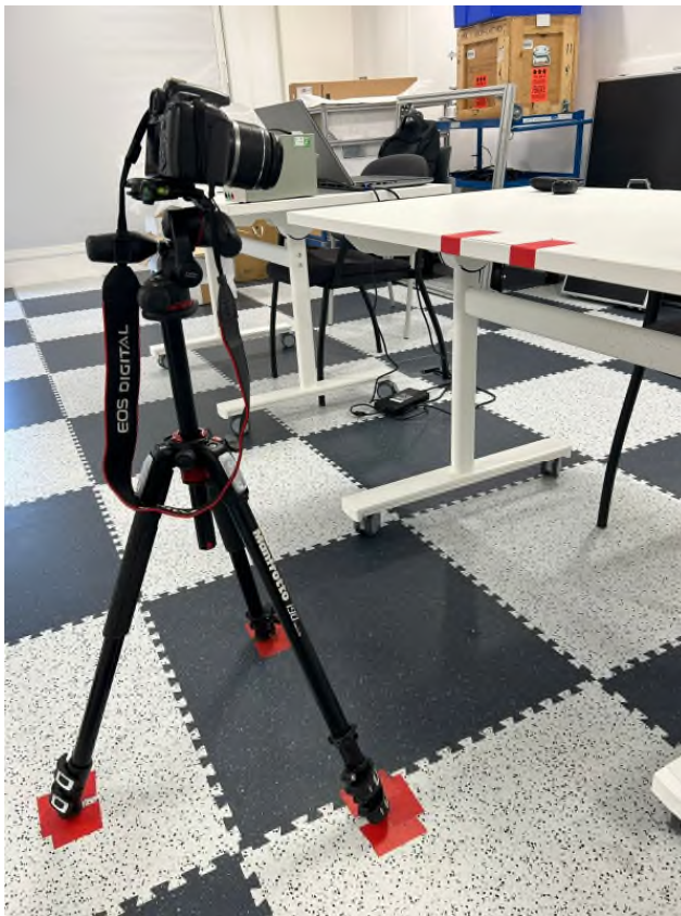
Figure 7: Camera setup for taking photos of the LiDAR front face.
