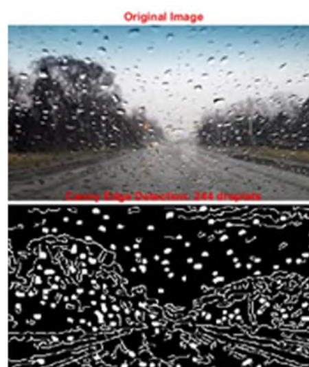
Figure 13: Canny Edge Detection more challenging example.
